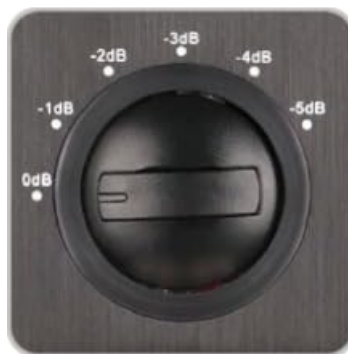
Image: A close-up of the treble adjust knob, showing attenuation options from 0dB to -5dB.
