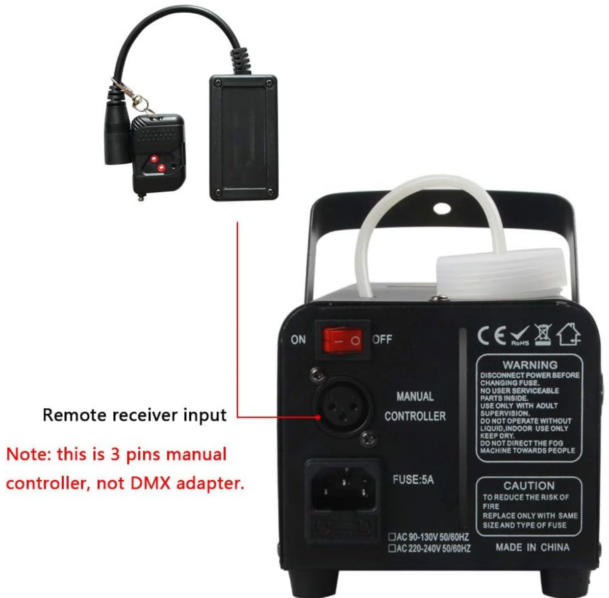
Figure 3: Example of a fog machine's 3-pin manual controller input, where the receiver should be connected. This is a manual controller, not a DMX input.
