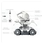
Figure 2: Exploded view of the Kokido Robot Manga X, illustrating its main components and internal accessory storage.
