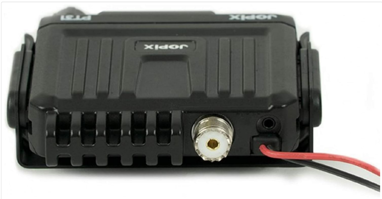
Image 5.1: Rear panel of the JOPIX PT31, illustrating the antenna connector and power input.
