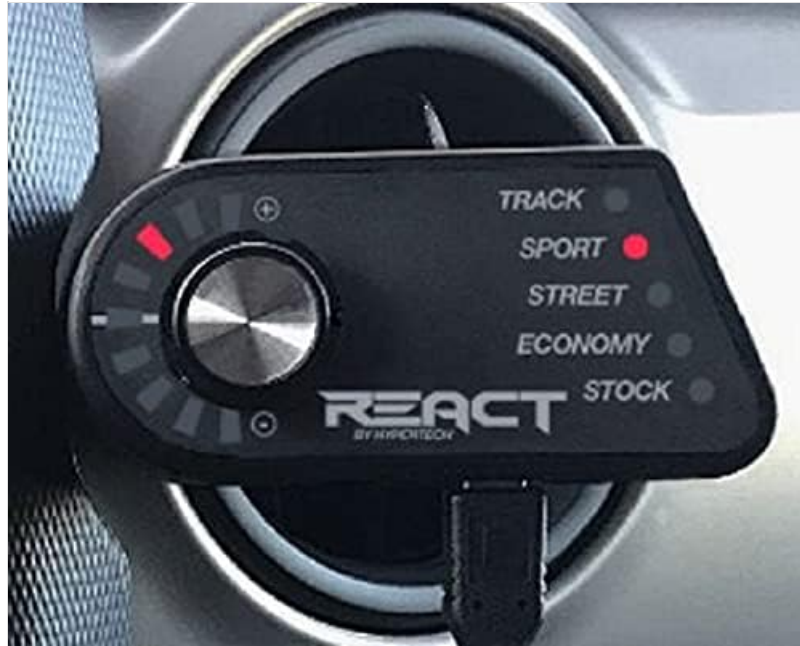
Image: Hypertech React control module installed on a vehicle's A/C vent, showing the display and control knob.
