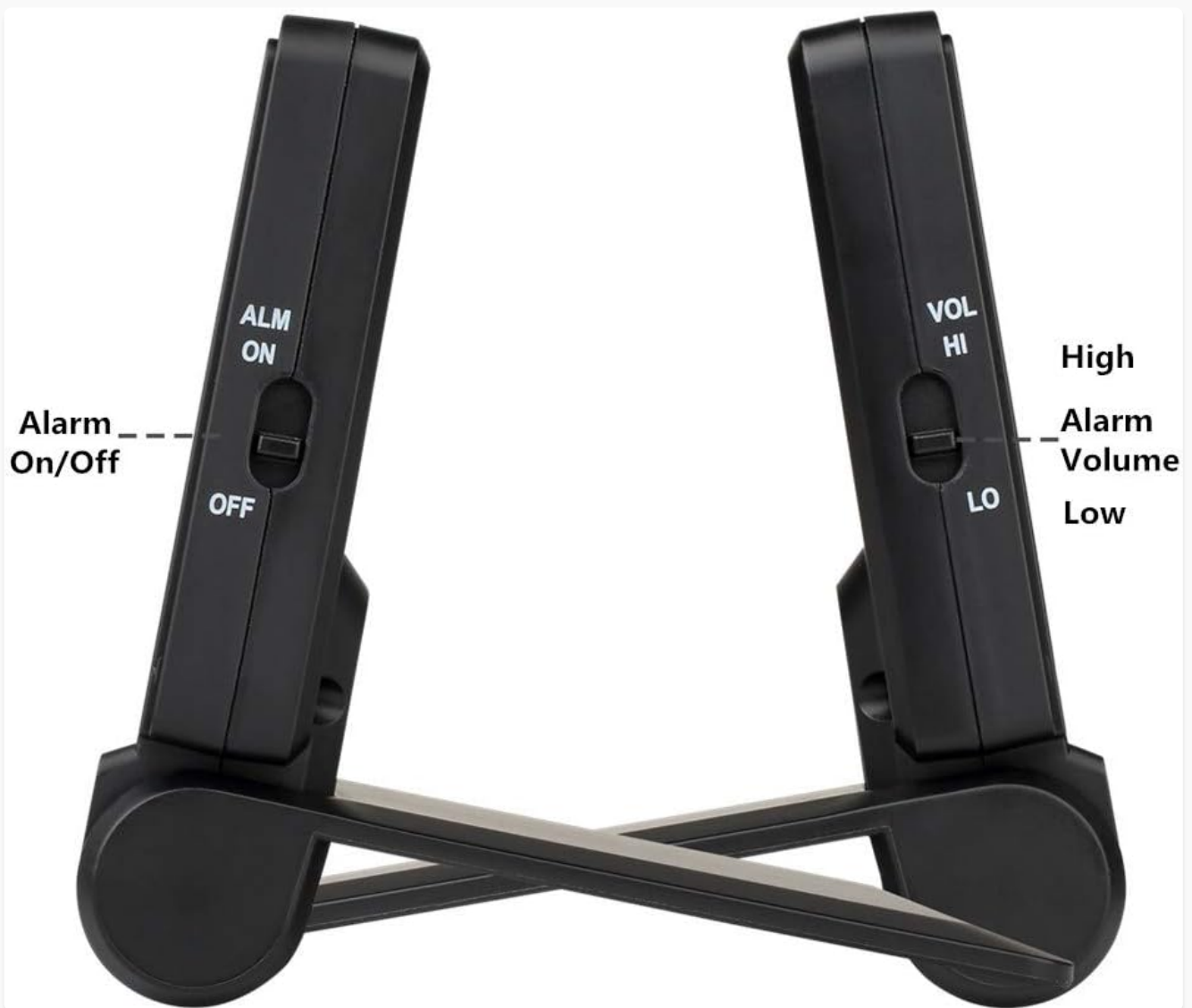
Figure 4: Side switches for alarm activation and volume.
