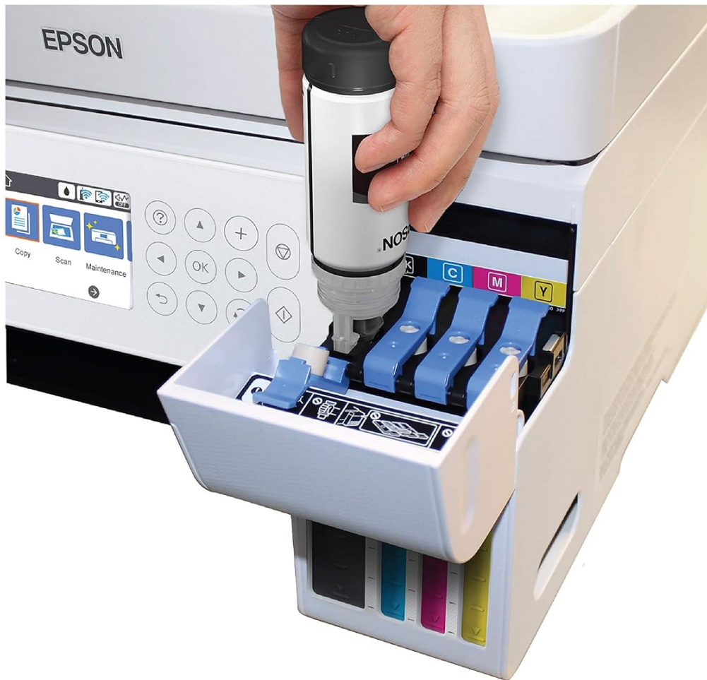
Figure 2: Illustration of filling ink tanks with EcoFit bottles. Each bottle is uniquely keyed to fit only the correct color tank, preventing accidental misfilling.
