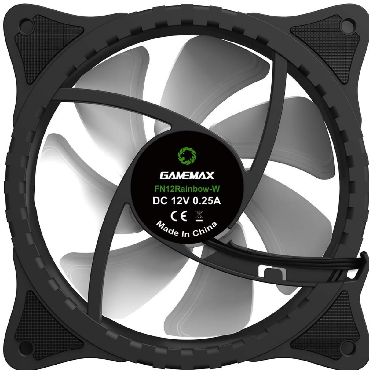
Image 8.1: Back view of the GameMax Mirage fan, displaying the product label with model and electrical specifications.
