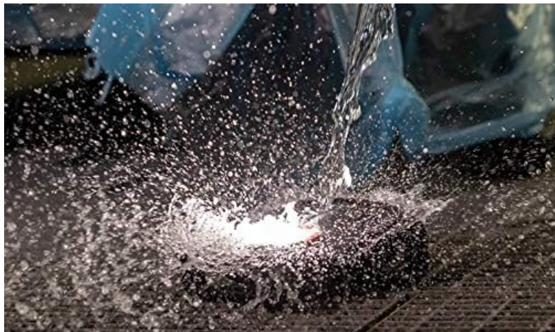
Scangrip light undergoing a water splash test, indicating its water-resistant design.
