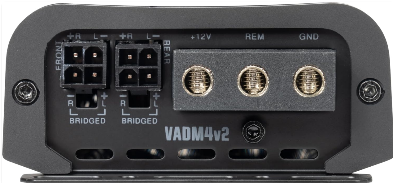
Figure 5: Close-up view of the power input and speaker output terminals on the NVX VADM4v2 amplifier. Connections include GND (Ground), REM (Remote Turn-On), +12V (Power), and speaker outputs for CH1-CH4.
