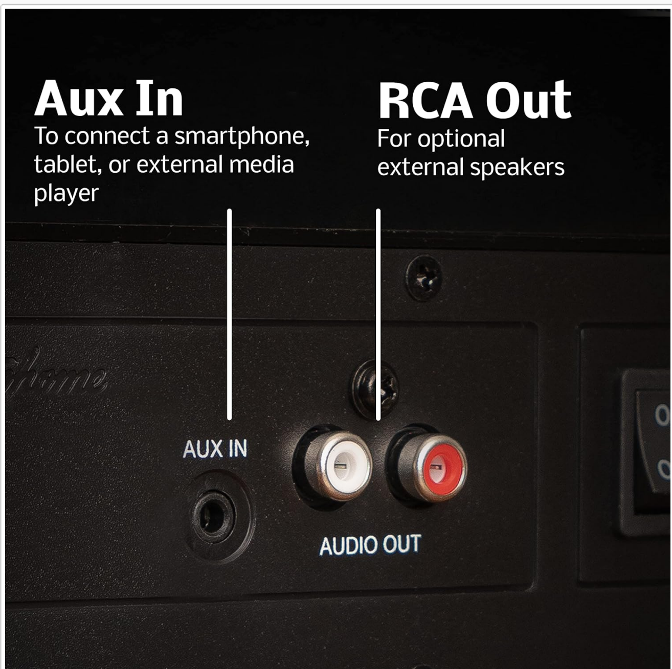
Image: A detailed view of the rear panel of the Electrohome Kingston RR75, highlighting the 'AUX IN' port for connecting smartphones or external media players, and the 'AUDIO OUT' (RCA) ports for optional external speakers.
