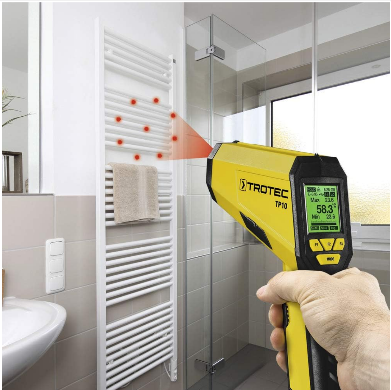
Figure 5: The TROTEC TP10 being used to measure the temperature of a radiator, illustrating a practical application of non-contact temperature measurement.
