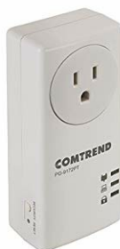
Figure 4: Side view of the Comtrend PG-9172PT Powerline Adapter, showing the Security/Reset button.
