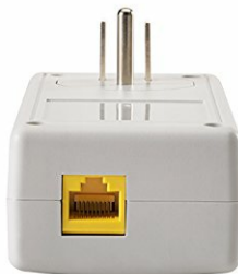
Figure 3: Bottom view of the Comtrend PG-9172PT Powerline Adapter, highlighting the Ethernet port.
