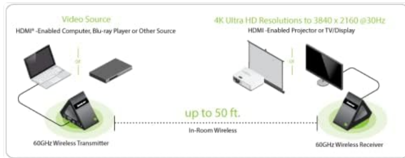
Image: A diagram illustrating the typical setup for the IOGEAR GW4K30GH60. It shows an HDMI-enabled computer or Blu-ray player connected to the 60GHz Wireless Transmitter, which then wirelessly transmits the signal up to 50 feet to the 60GHz Wireless Receiver, connected to an HDMI-enabled projector or TV/display, supporting 4K Ultra HD resolutions up to 3840 x 2160 @ 30Hz.
