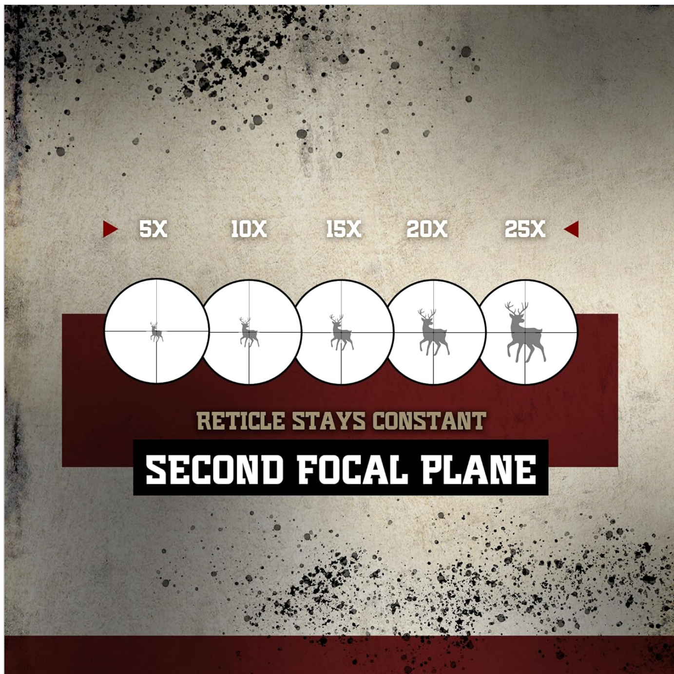
Figure 3.2: Illustration of the Second Focal Plane reticle, demonstrating how the reticle size remains constant relative to the field of view across different magnifications.
