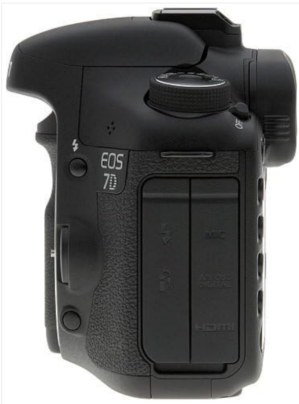
Figure 4: Left side view of the Canon EOS 7D, revealing the port covers for audio, USB, and HDMI connections.
