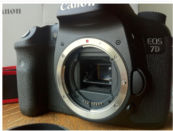
Figure 6: Close-up of the Canon EOS 7D lens mount, with the camera sensor visible.
