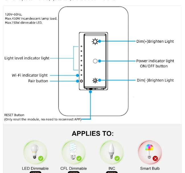
Image Description: This diagram illustrates the various parts of the Nexete Smart Wi-Fi Dimmer Switch. It shows the Dim(+) button for brightening, the Dim(-) button for dimming, the Power ON/OFF button, the Wi-Fi indicator light, the light level indicator lights, and the RESET button. The diagram also indicates compatibility with LED Dimmable (150W), CFL Dimmable (150W), and INC (400W) bulbs, while explicitly stating incompatibility with Smart Bulbs.
