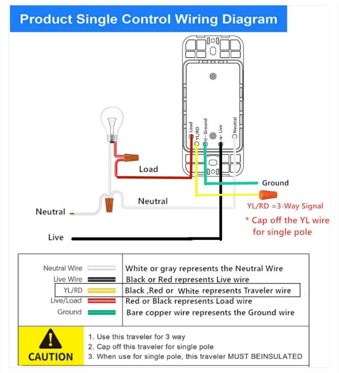
Image Description: This diagram illustrates the wiring for a single-pole setup of the Nexete Smart Wi-Fi Dimmer Switch. It shows connections for Live (black), Neutral (white), Load (red/black), and Ground (green) wires. The YL/RD (traveler) wire should be capped off and insulated for single-pole use. A caution advises to use this product with a 4A circuit breaker upstream.
