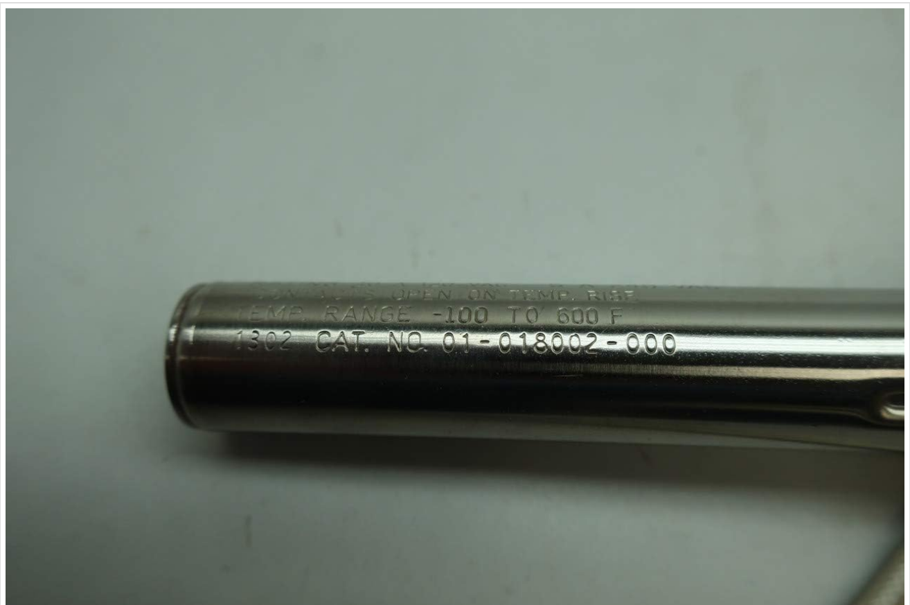
Figure 2: Close-up view of the THERMOSWITCH body, indicating a temperature range of -100 to 600 F and Cat. No. 01-018002-000. The marking 'OPEN ON TEMP. RISE' specifies its operational characteristic.
