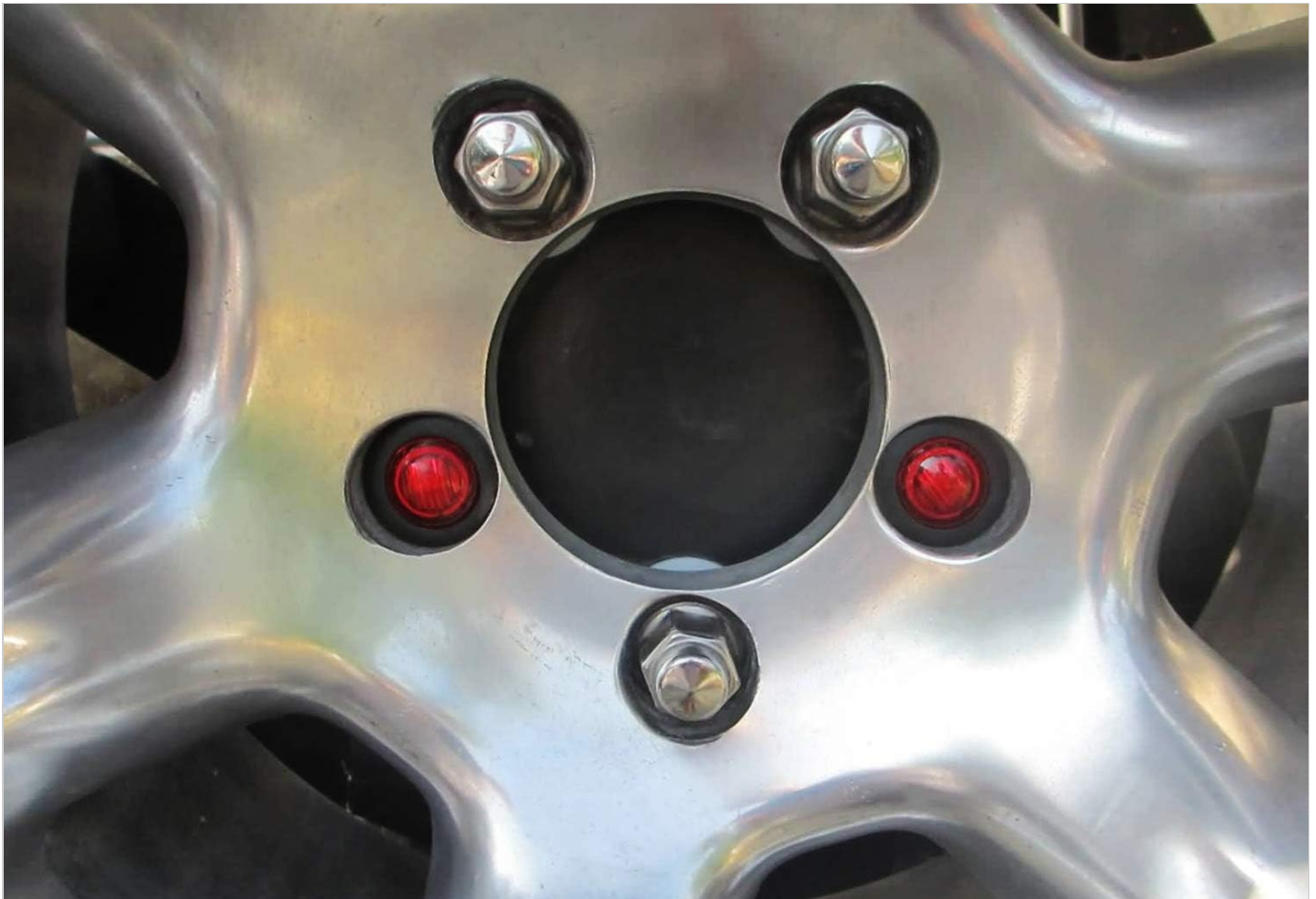
The LED lights inserted into the lug nut holes of a spare tire wheel.
