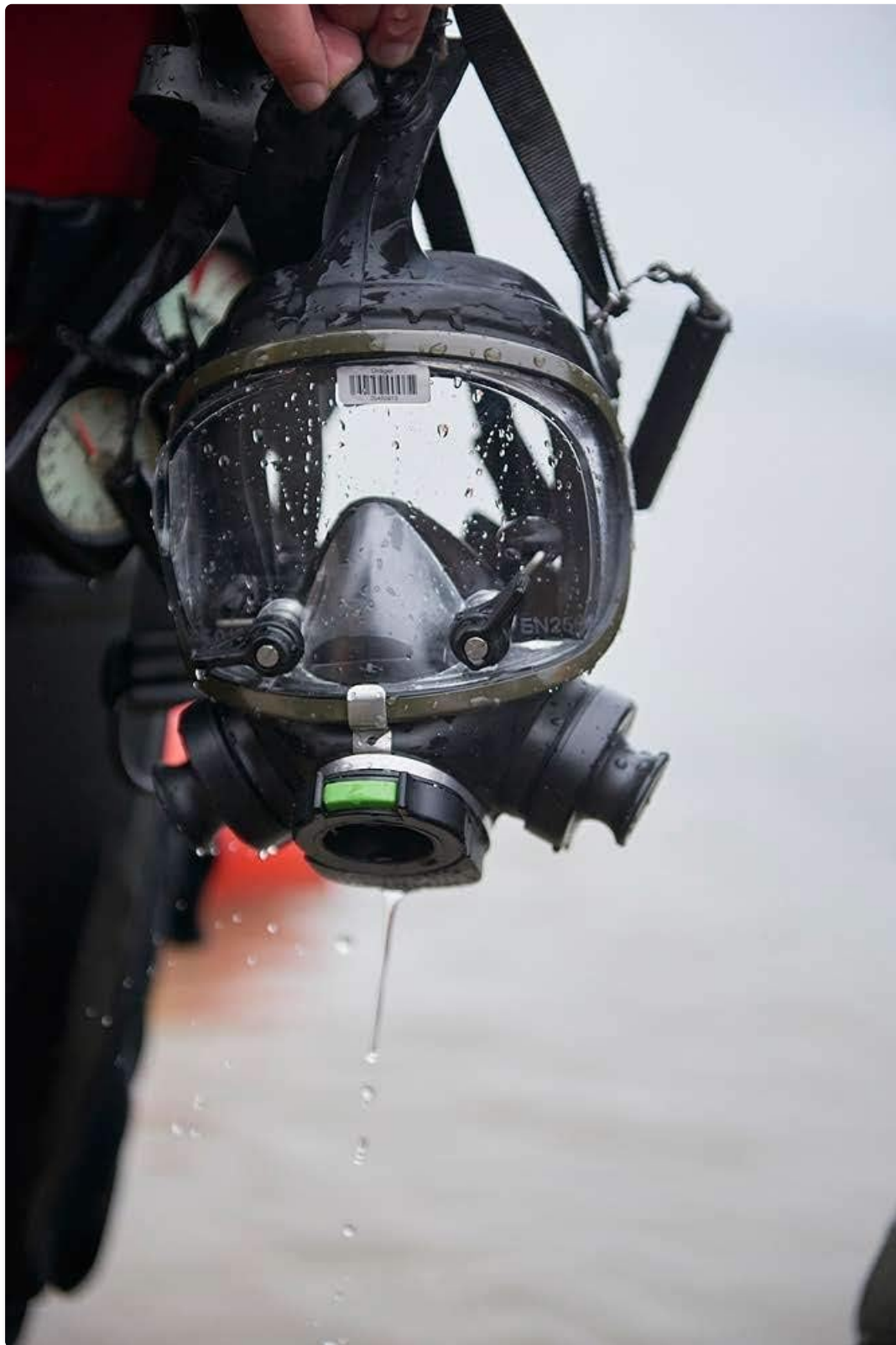
Figure 6.1: The mask after use, showing water dripping, indicating the need for rinsing.
