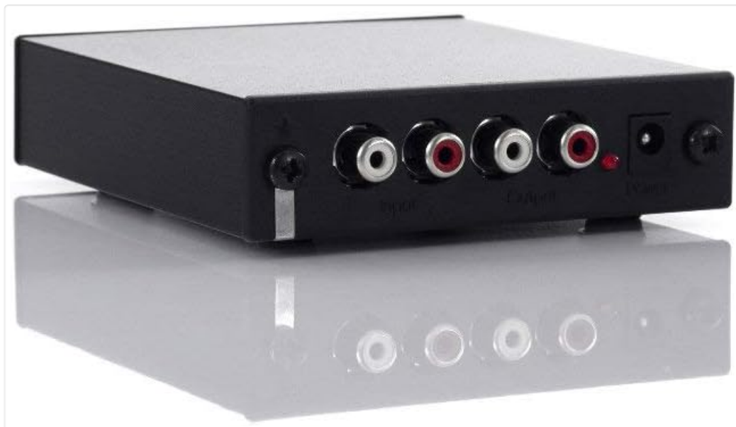
Figure 3: Rear panel connections of the Rega Fono Mini A2D Mk2. This image shows the RCA 'Input' and 'Output' jacks, the 'Power' input, and the ground terminal.
