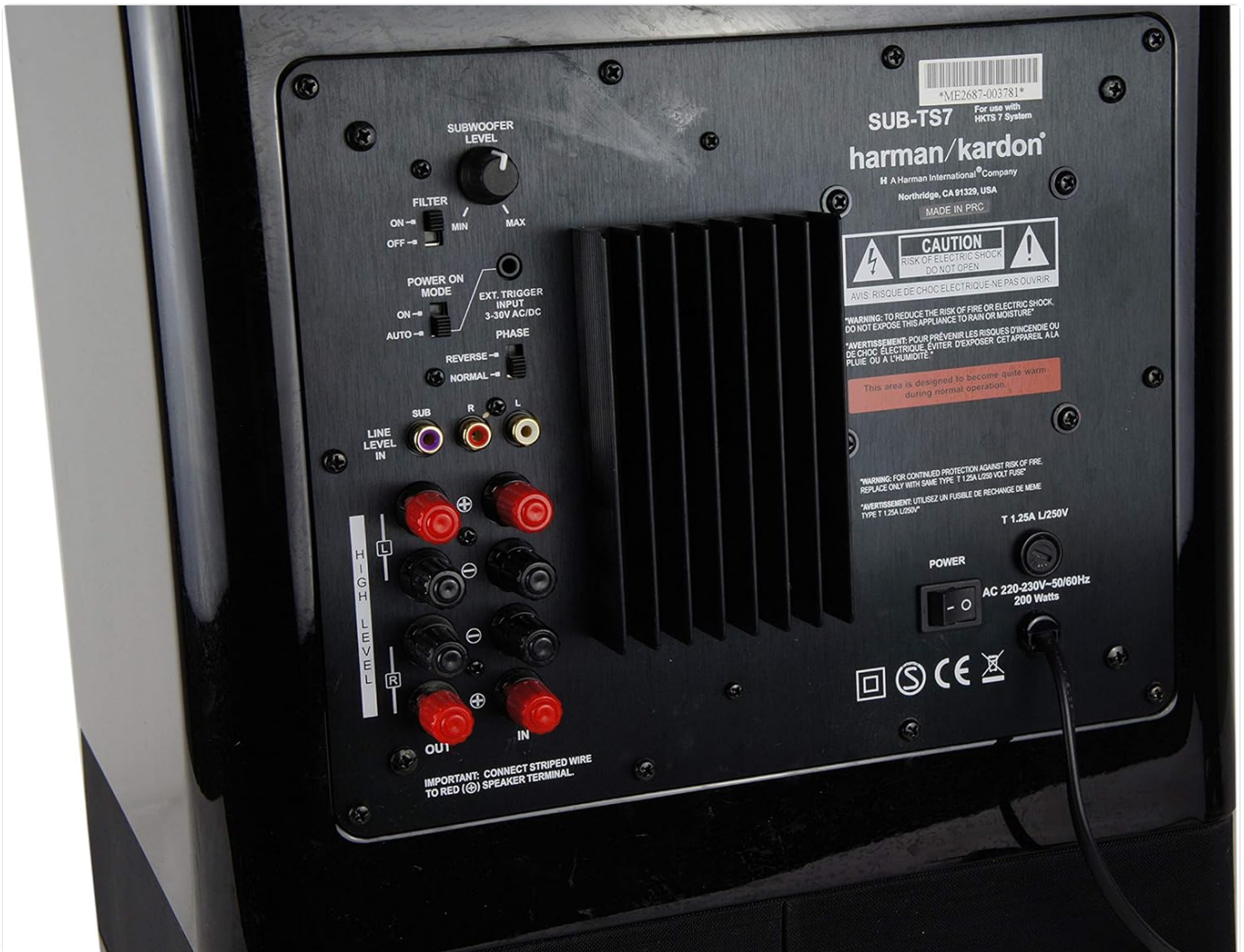
Figure 4: Detailed view of the rear control panel, including Subwoofer Level, Filter, Power On Mode, Phase, Line Level inputs, High Level inputs, and power connection.
