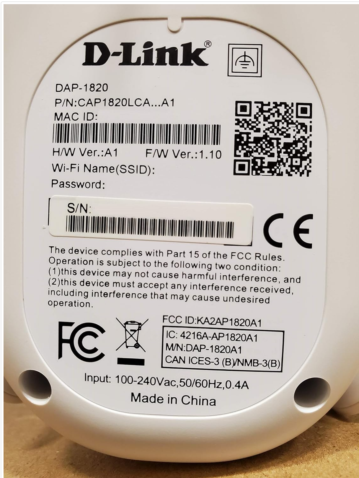
Figure 3.2: Back Label with Device Information
