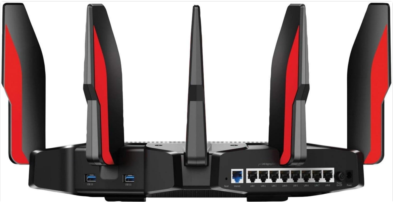
Figure 2.2.2: Rear View of Archer C5400X Router. This image shows the rear panel of the Archer C5400X, detailing its connectivity options. From left to right, it includes two USB 3.0 ports, a Reset button, the Internet (WAN) port, eight Gigabit LAN ports (LAN1-LAN8), a Wi-Fi On/Off button, and the Power On/Off button. The Link Aggregation feature is indicated above LAN ports
