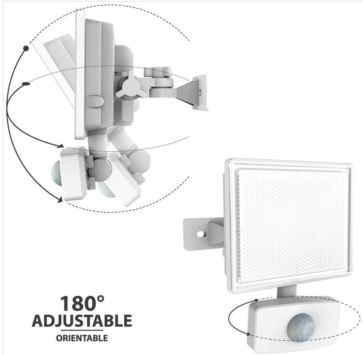
The projector head and the motion detector are both adjustable. You can orient the light and the sensor up to 180 degrees to cover your specific area. Loosen the adjustment screws, position the light and sensor as desired, and then tighten the screws to secure them.
