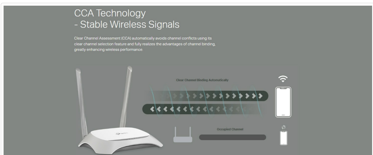
Figure 5.1: Diagram illustrating CCA Technology, which helps in selecting clear channels to improve wireless signal stability and performance.
