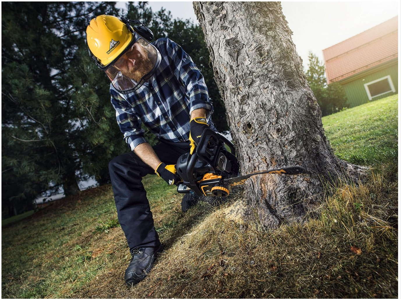
Figure 4: A user wearing full safety gear, including a helmet with face shield and ear protection, operating the McCulloch CS 42STE chainsaw near the base of a tree. This emphasizes safe operating practices.
