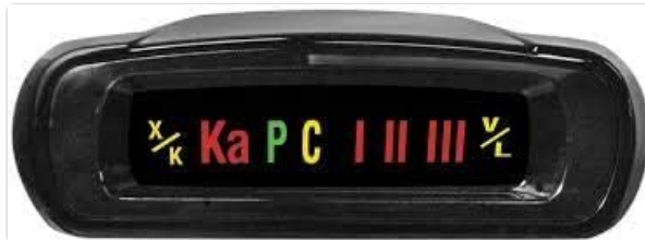
Figure 3: Close-up view of the Whistler Z-11R+ icon display, showing indicators for X, K, Ka bands, and signal strength bars.
