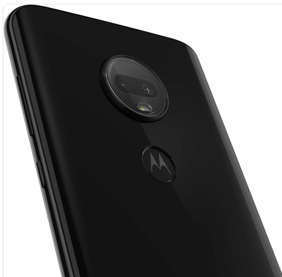
Image 2: Rear view of the Moto G7, highlighting the 12MP + 5MP dual camera setup with LED flash and the integrated fingerprint sensor for secure unlocking.
