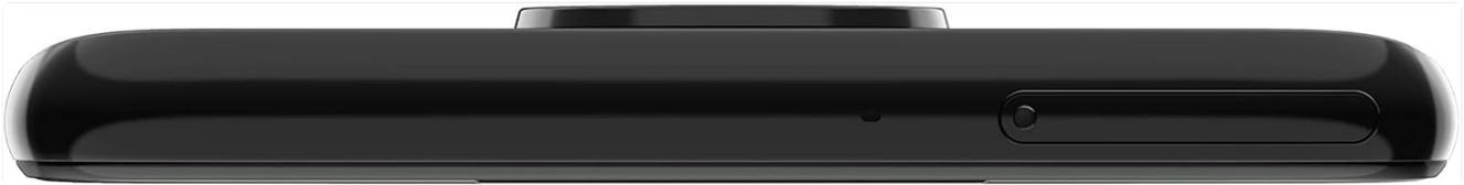
Figure 2.2: Top edge of the Moto G7, illustrating the location of the SIM tray.
