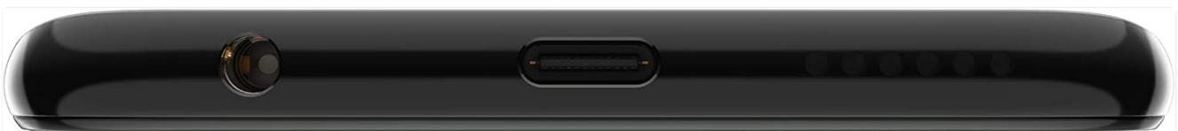
Figure 2.4: Bottom edge of the Moto G7, highlighting the USB-C charging port and 3.5mm audio jack.
