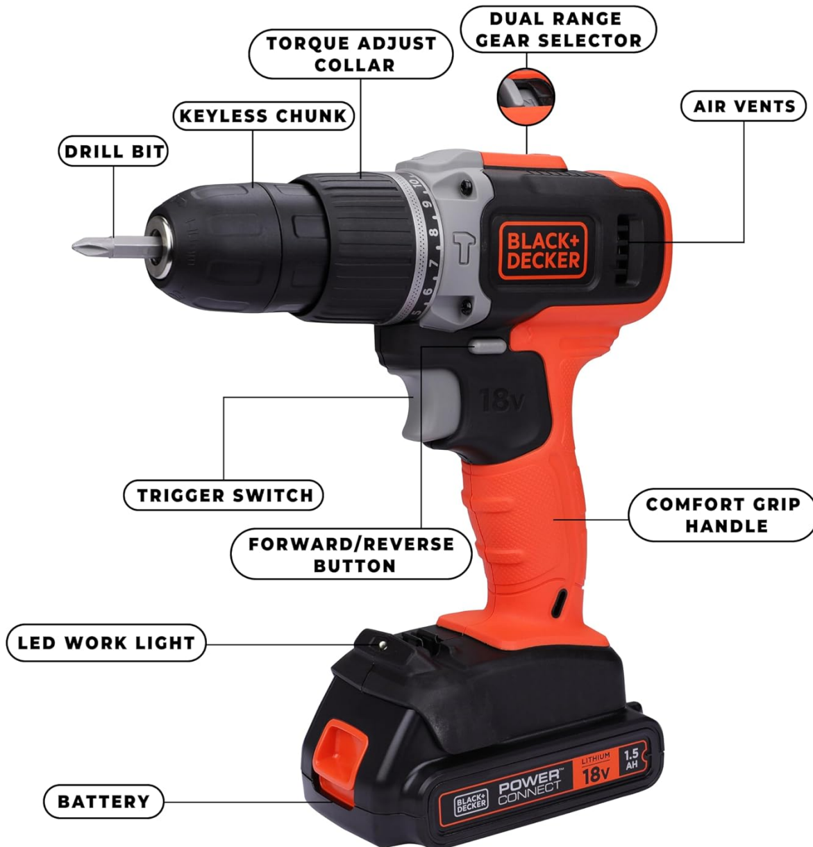
Figure 2: Labeled diagram of the BLACK+DECKER BCD003C1 Cordless Hammer Drill Machine, highlighting parts such as the drill bit, keyless chuck, torque adjust collar, dual range gear selector, air vents, trigger switch, forward/reverse button, comfort grip handle, LED work light, and battery.
