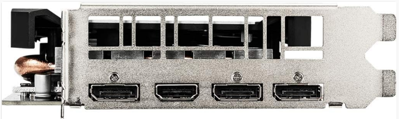
Figure 3.2: Rear view of the graphics card, illustrating the three DisplayPort (v1.4) outputs and one HDMI (2.0b) output for connecting to various display devices.
