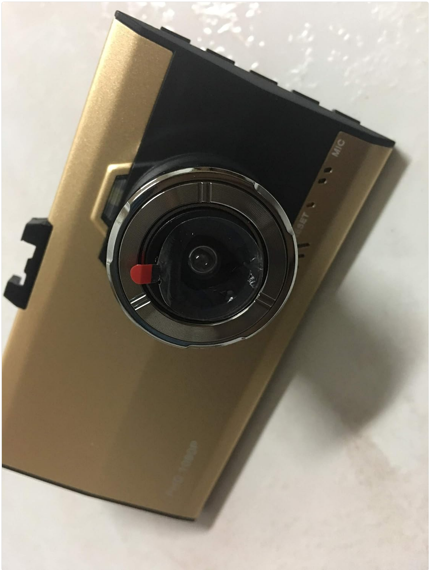
Image: Top-down perspective of the dash cam, providing a clearer view of the camera lens and the microphone (MIC) input. This angle also shows the mounting slot at the top.
