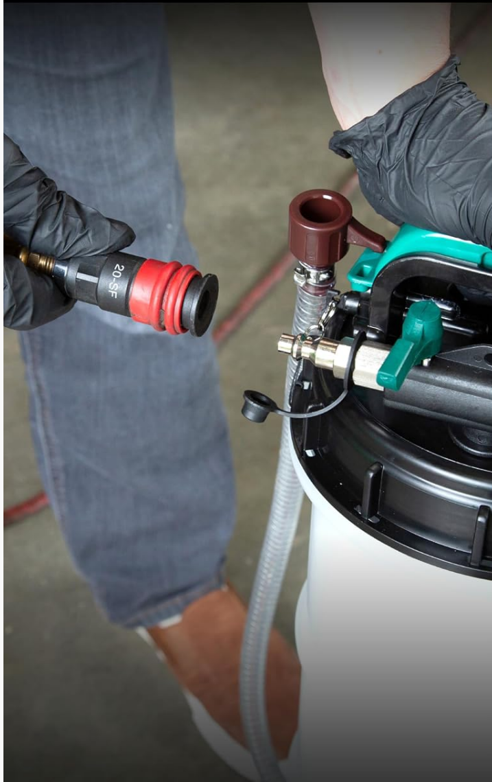
Image: Demonstrates the two modes of operation: pneumatic connection on the left and manual pumping on the right.
