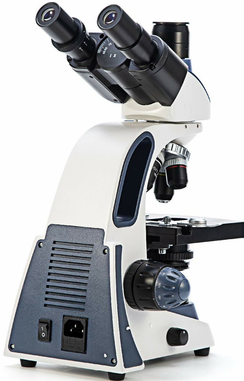
Figure 8: Coarse and fine focus adjustment knobs.
