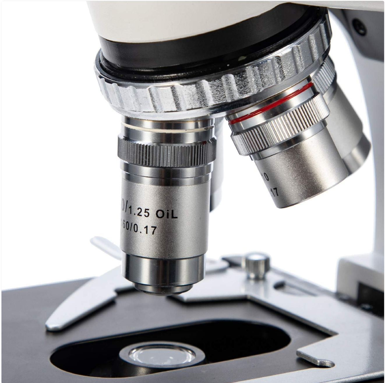
Figure 6: A detailed view of the objective lenses mounted on the revolving nosepiece.
