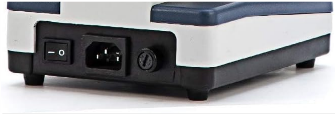
Figure 4: Rear view of the microscope, highlighting the power input and switch for operation.
