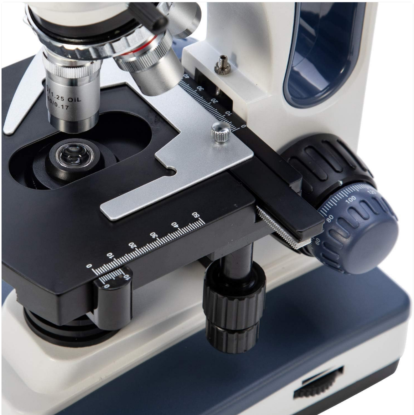
Figure 5: A close-up view of the mechanical stage, showing the slide holder and X-Y translational axis controls.
