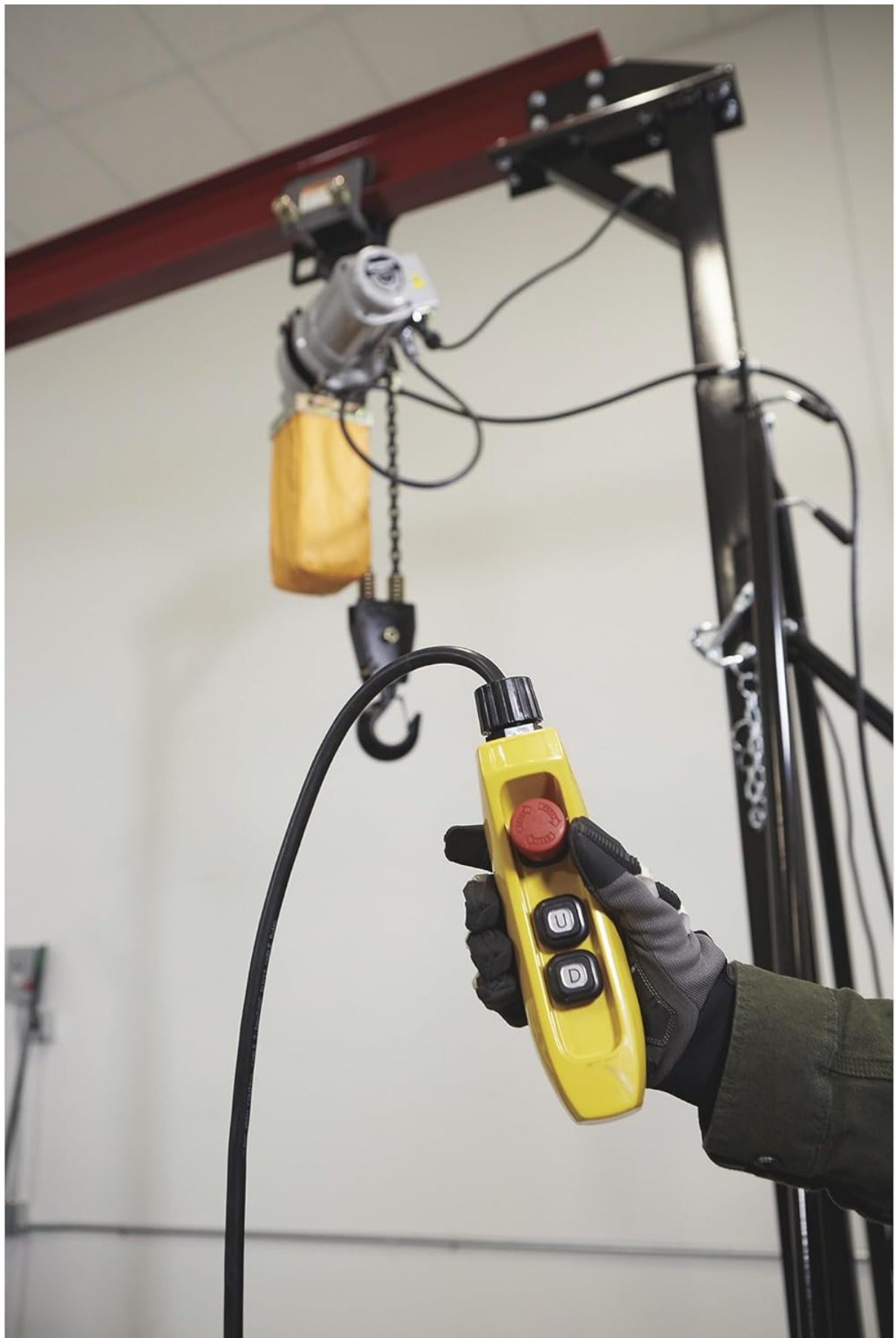
Figure 5.1: The handheld remote control with clearly marked 'UP', 'DOWN', and 'EMERGENCY STOP' buttons.
