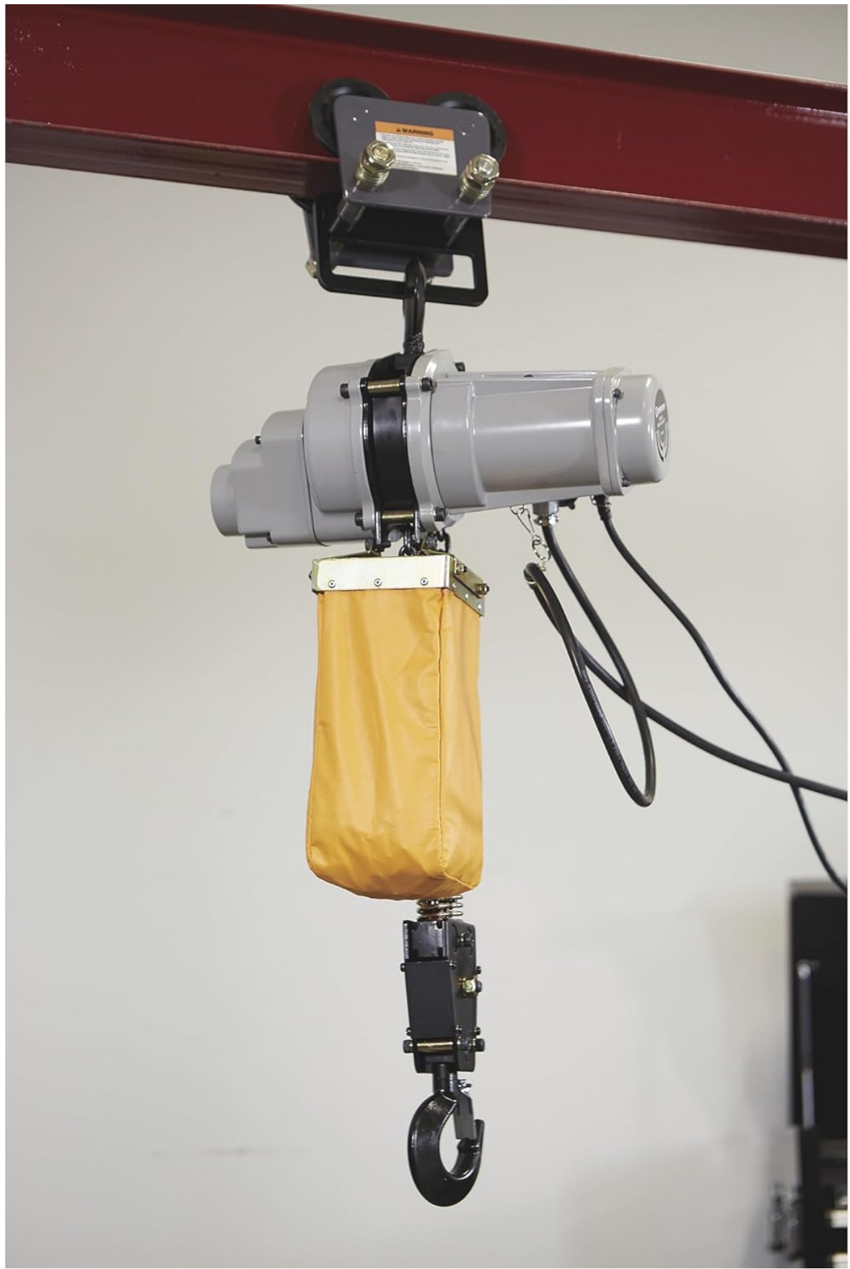
Figure 4.1: The electric hoist securely installed on an overhead beam, ready for operation.
