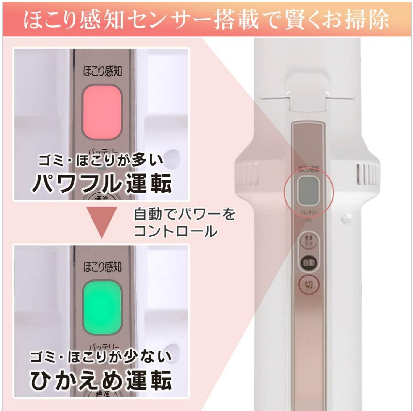
Image 3: The dust sensor indicator. Red indicates high dust levels and powerful operation, while green indicates low dust levels and reduced power operation, conserving battery.
