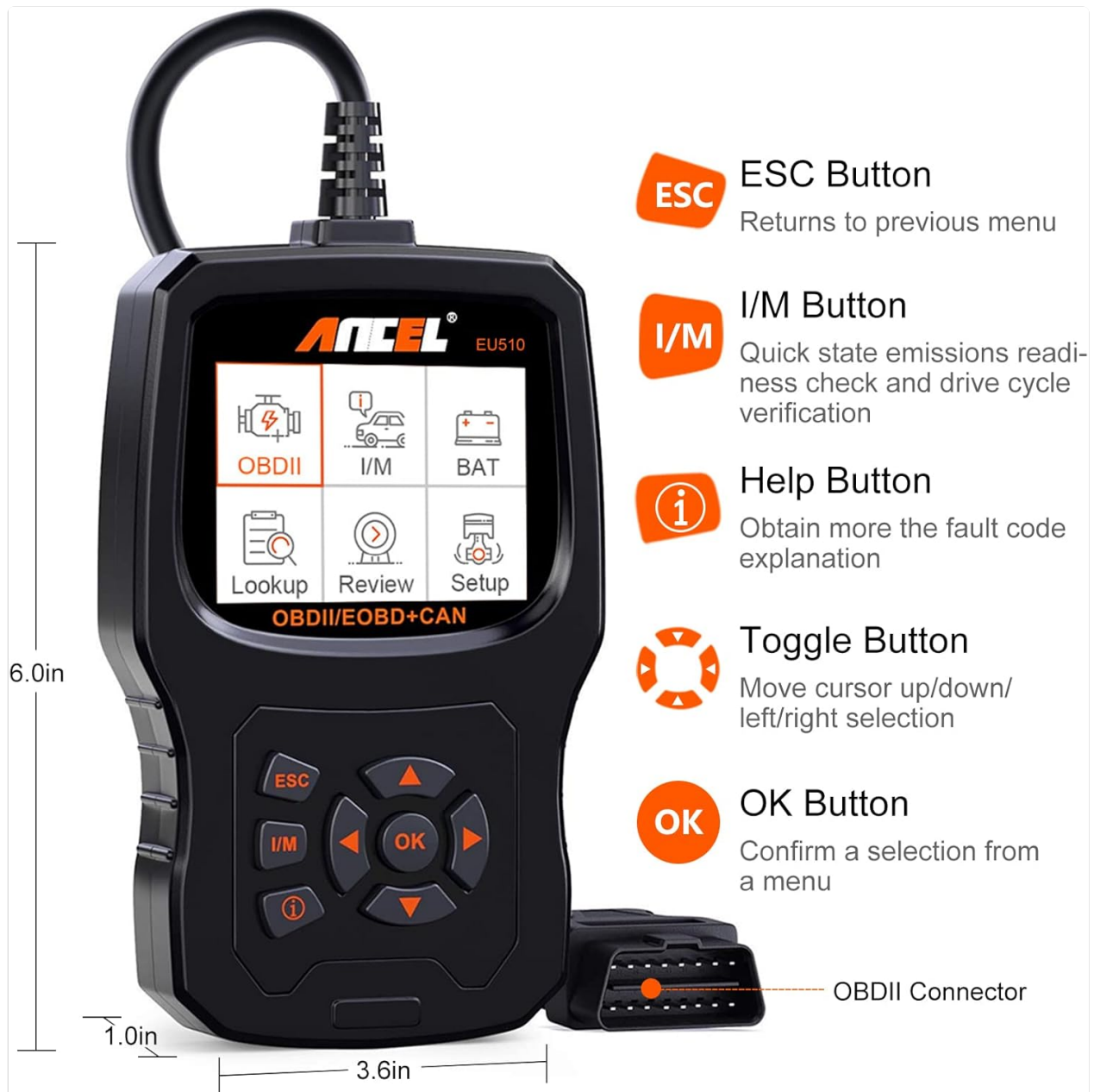
Figure 2.1: Detailed view of the ANCEL EU510, highlighting its buttons and approximate dimensions.
