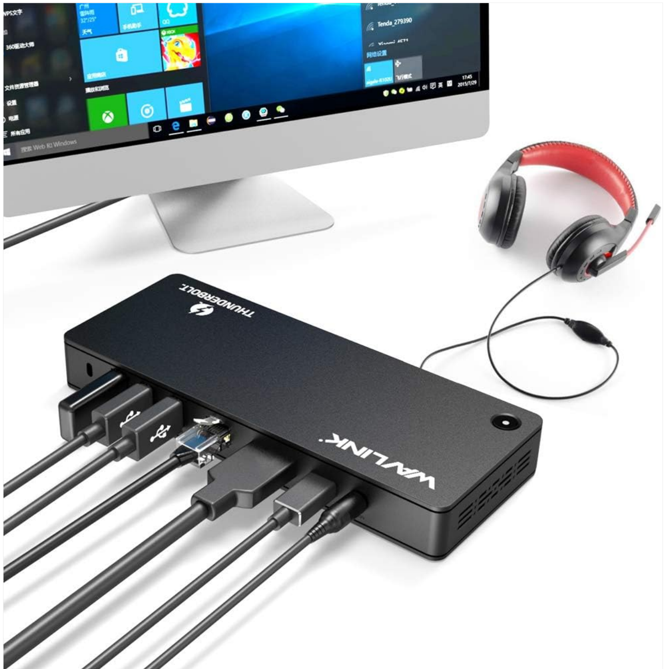
Image 4: Rear panel of the docking station, displaying the Lock slot, three USB 3.0 ports, Gigabit Ethernet port, DisplayPort, a second Thunderbolt 3 port (40Gbps), and the DC 20V power input.
