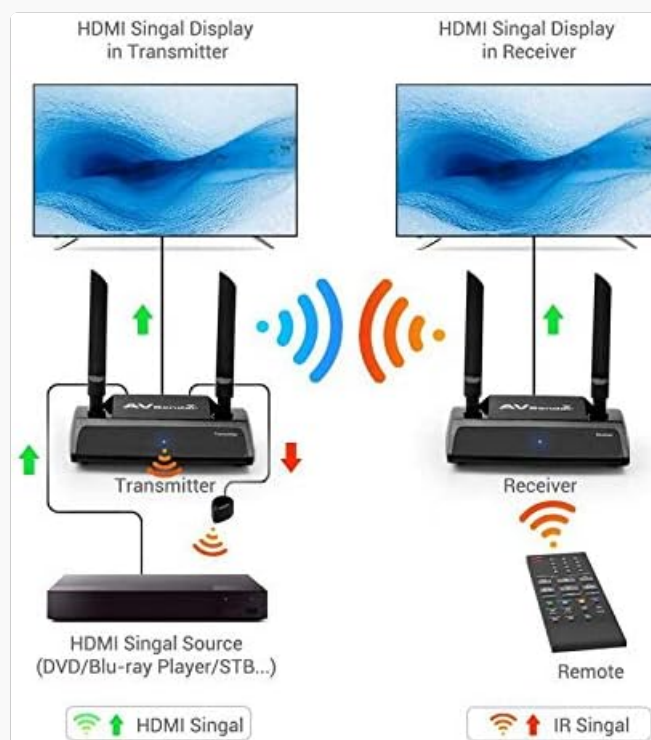
Image 3.2: Diagram illustrating the connection flow from an HDMI signal source to the transmitter, and wirelessly to the receiver and a remote display, including IR remote control setup.
