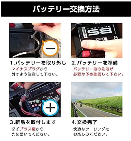
Figure 3: Step-by-step visual guide for battery replacement, emphasizing correct terminal connection order.
