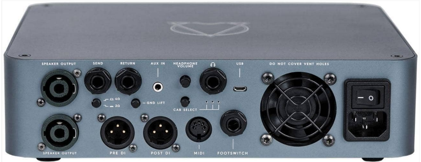
Figure 2.2: Rear panel of the Alpha Omega 900 Bass Head, detailing speaker outputs, effects loop, auxiliary input, headphone output, USB, DI outputs, MIDI, and footswitch connections.
