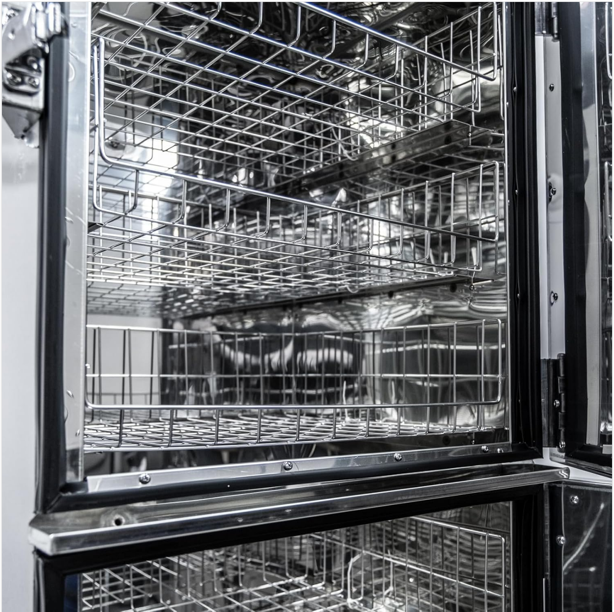
Figure 2: Interior racks for towel loading.
