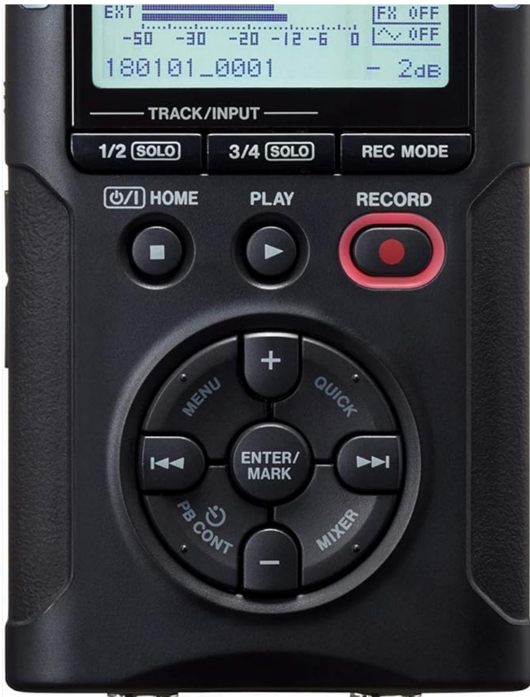
Figure 1.1: Front view of the TASCAM DR-40X, showing the adjustable microphones, display, and control buttons.
