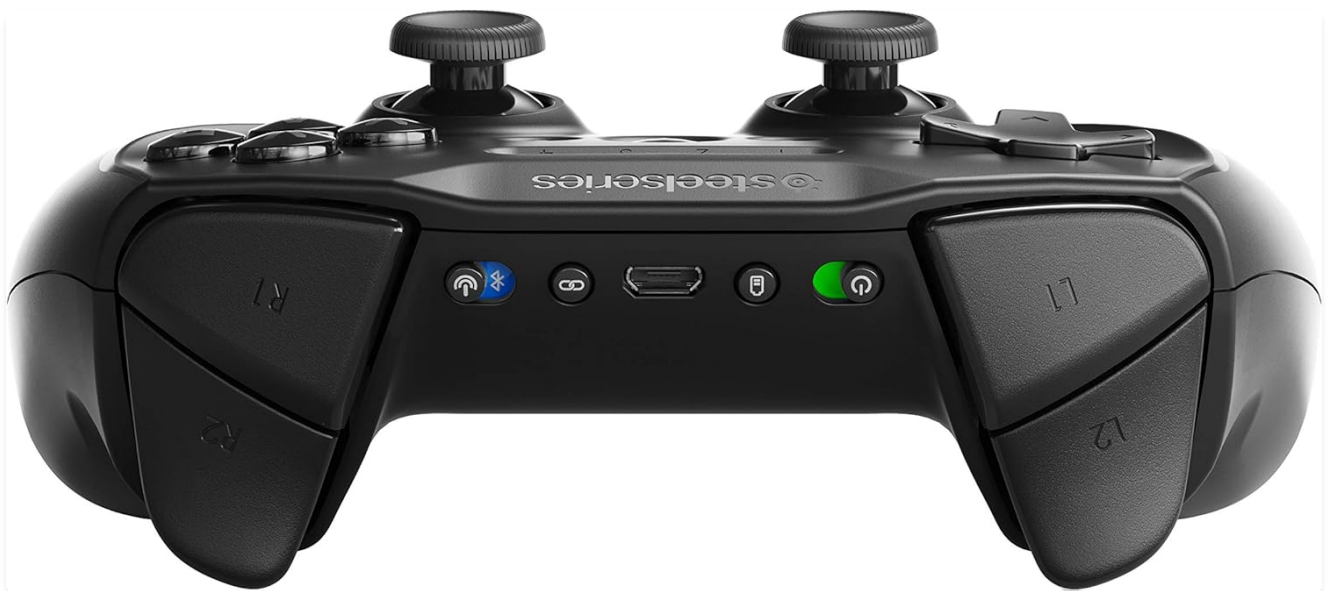
Figure 2: Bottom view of the controller, highlighting the micro-USB charging port and the wireless mode switch.
