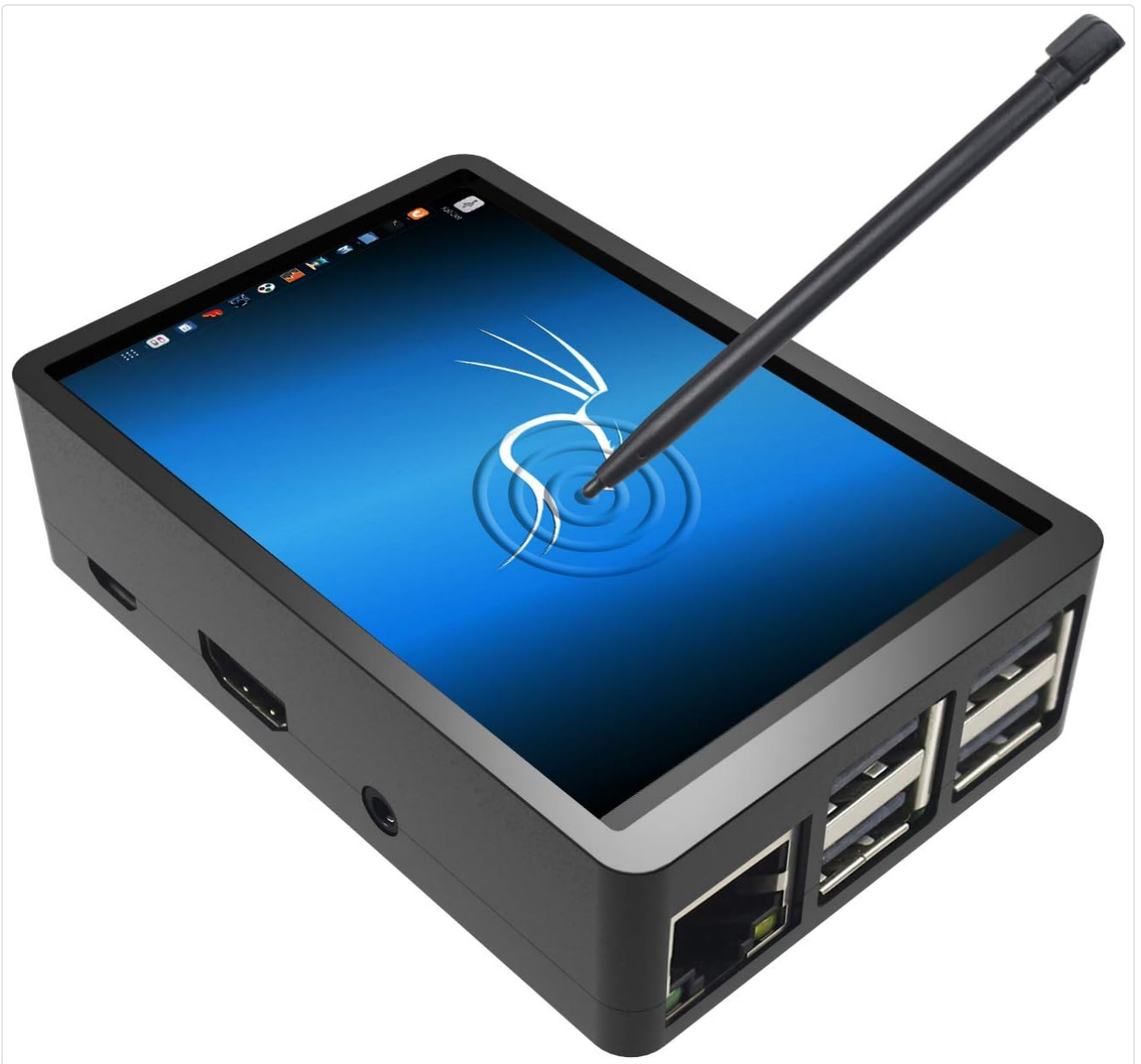
Image: Fully assembled Raspberry Pi with the 3.5-inch touch screen integrated into its protective case, shown with a stylus.
