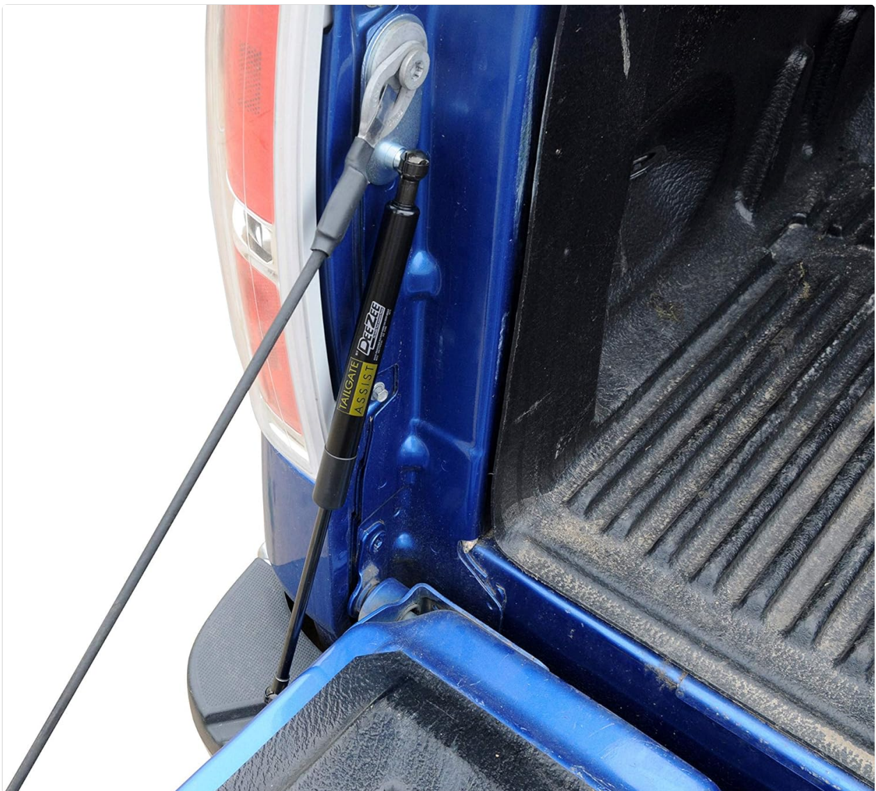
Figure 3.1: Close-up of the Dee Zee Tailgate Assist shock damper installed on the truck bed side, connected to the tailgate.
