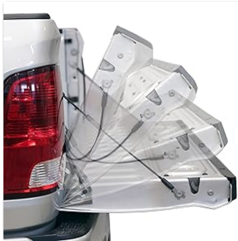
Figure 3.3: Visual representation of the tailgate's smooth, controlled descent with the assist in action.
