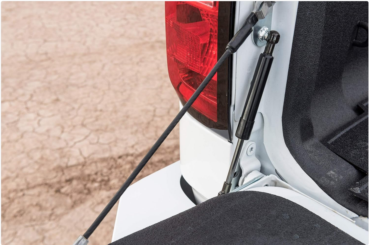
Figure 3.1: Close-up of the Dee Zee Tailgate Assist shock damper installed on the truck bed side, connected to the tailgate.
