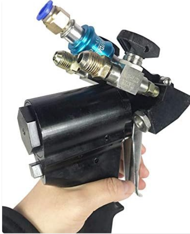
Figure 4: Top view of the spray gun, highlighting the air and material inlet connections and the nozzle assembly.
