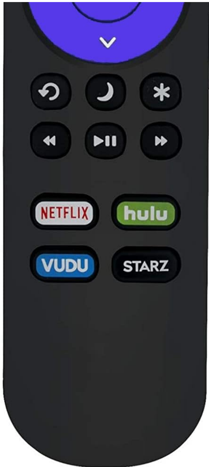
Figure 1: Front view of the USARMT 101018E0011 remote control, showing all buttons including the power, navigation, playback, and dedicated streaming service buttons (Netflix, Hulu, Vudu, Starz).
